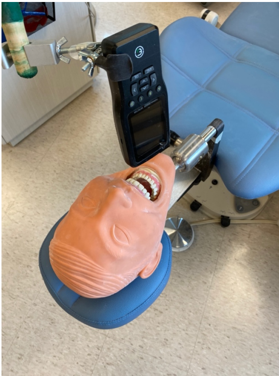
Figure 1. Debonding set-up for positive control, no evacuation system
