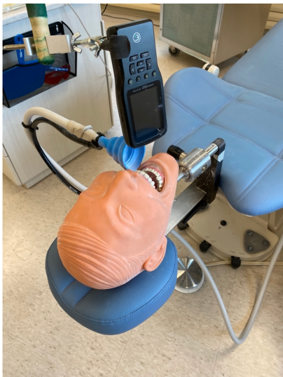
Figure 4. Debonding set-up for A-HFHVE
